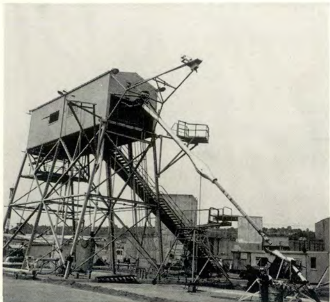
With the coming of the KC-135, Boeing's jet tanker, a new, high-speed refueling boom was needed. Before installation and in-flight tests, the equipment shown here gave engineers data on design deficiencies.
