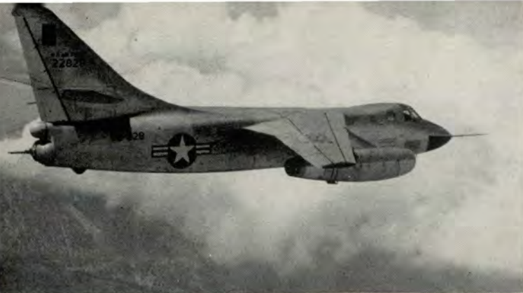
The B-66 is a stable aircraft with good control responses. It is equipped with in-flight refueling facilities for increased range.
