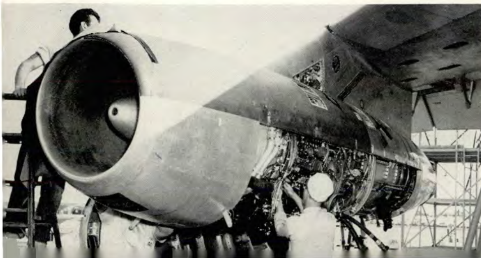
The J-71-11 engines are meeting the thrust guarantees. Low slung, they are readily accessible.
