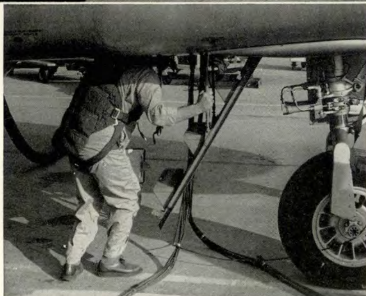
The aircraft is built fairly close to the ground and entrance can be made through a hatch on the under-side of the fuselage. Below, the starting unit is hooked to a single point receptacle.
