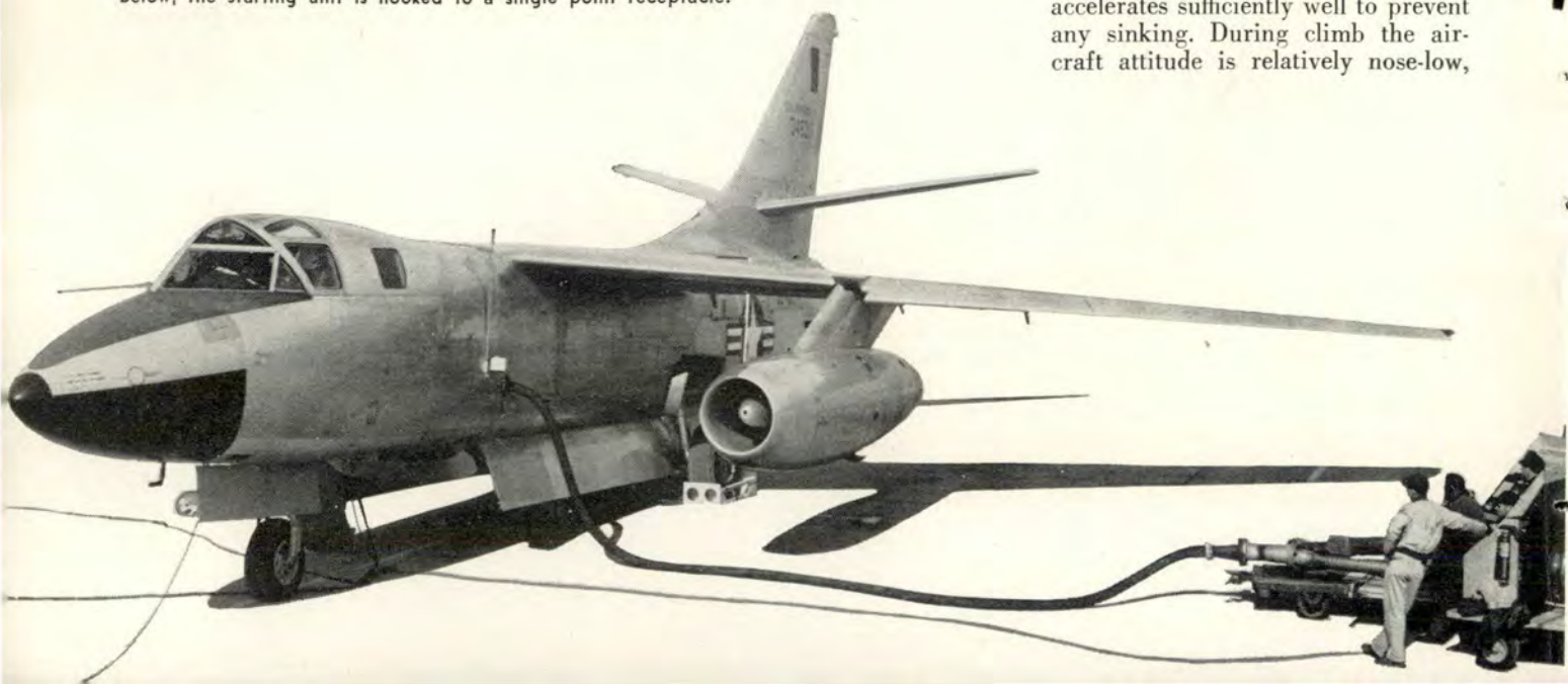
The aircraft is built fairly close to the ground and entrance can be made through a hatch on the under-side of the fuselage. Below, the starting unit is hooked to a single point receptacle.
