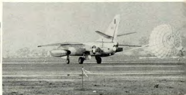
Consistently good landings can be made by use of normal landing techniques. Drag chute reduces the landing roll.
