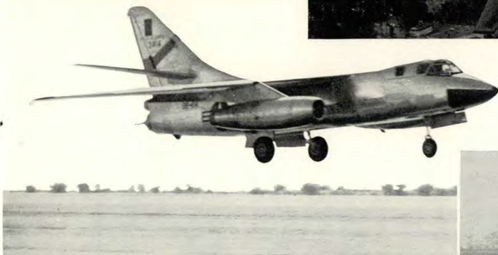
Consistently good landings can be made by use of normal landing techniques. Drag chute reduces the landing roll.
